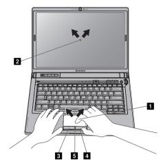
The blue indicator 5 is lit when the touch pad is activated, when the touch pad is disabled with Fn + F8, the indicator will be off.
